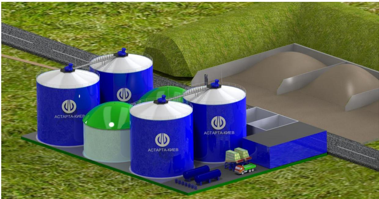
The capacity of the biogas facility is 1,200 tonnes of processed bagasse and 150,000 cu m of produced biogas a day. The biogas consists of 53 percent methane, 46 percent CO<sub>2</sub> and 1 percent other gases (O<sub>2</sub>, N<sub>2</sub>).
